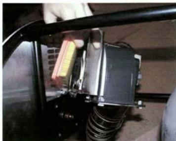
Figure 4. Filter Under Blower
