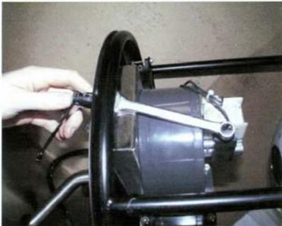
Figure 3. Removing the Blower
